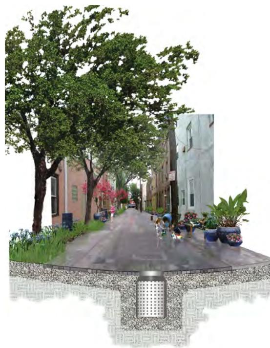
Potential green stormwater infrastructure for alleys to improve on-site stormwater quality from the Green City Clean Water Long-Term CSO Control Plan
